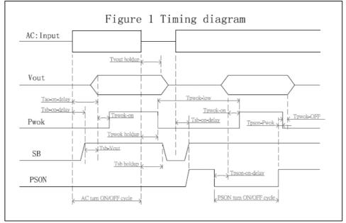
These are the timing requirements for power supply operation including alone module outputs and multi model outputs. All outputs shall rise and fall monotonically.
